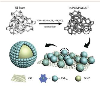
Fig. 1 Schematic illustration of PPGN
