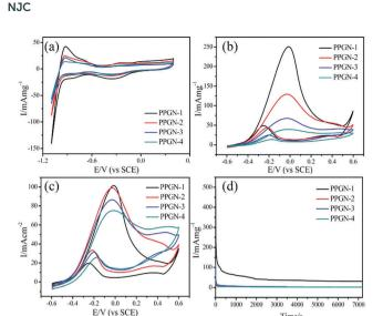
Fig. 5 CV curves of PPGN-n in 0.1 mol L<sup>-1</sup> KOH solution (a) and in 1 mol L<sup>-1</sup>  ${\rm CH_3OH}$  + 0.1 mol  ${\rm L^{-1}}$  KOH solution (b and c). The Chronoamperometry of PPGN-n in 1 mol L<sup>-1</sup> CH<sub>3</sub>OH + 0.1 mol L<sup>-1</sup> KOH solution (d).
