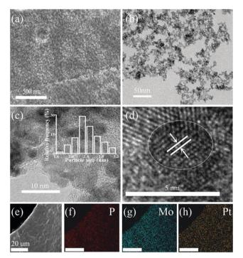
Fig. 2 The SEM (a), TEM (b) and HRTEM (c and d) of PPGN-1 and the corresponding elemental mapping of P, Mo and Pt (e-h).
