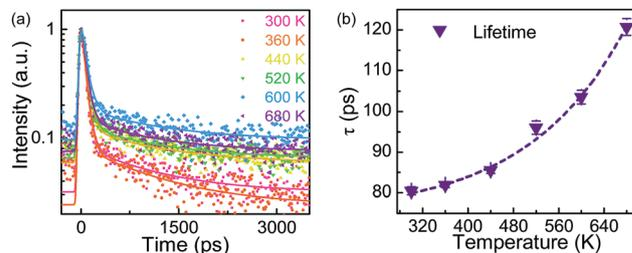
Fig. 5 (a) Time-resolved PL spectra of the  $K \rightarrow K$  direct emission at different temperatures. The solid lines are exponential decay fittings of the obtained experimental data points, giving out the effective fluorescence lifetime of the  $K \rightarrow K$  direct emission. (b) The fitted effective lifetime  $\tau$  as a function of the measurement temperature.
