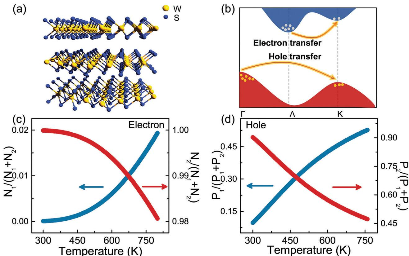
Fig. 1 (a) Structural schematic diagram of a multilayer 2H- $\text{WS}_2$  sample. (b) A scheme showing the transfer process of photo-carriers among different energy valleys and hills; the orange arrows indicate the transfer direction from  $\Lambda/\Gamma$  to K. Population ratio of the electrons (c) and holes (d) in the K point (blue curve) and the  $\Lambda/\Gamma$  point (red curve) as a function of the measurement temperature in ML- $\text{WS}_2$ .
