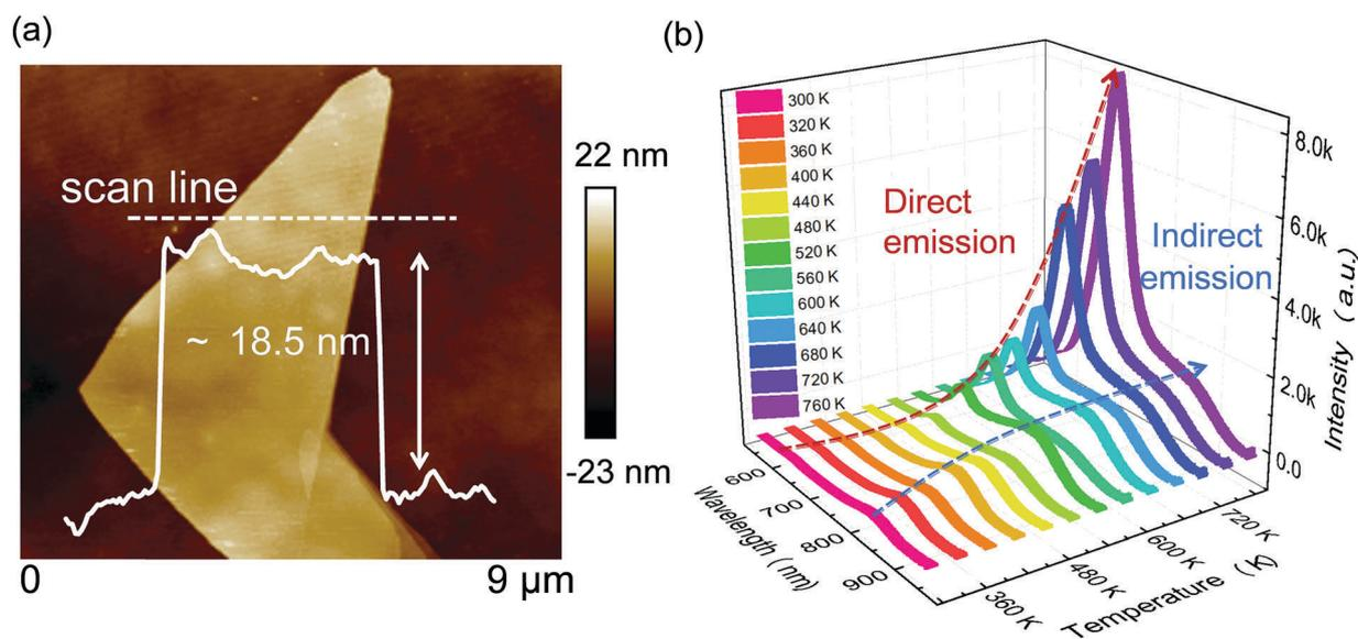
Fig. 2 (a) A typical AFM image showing the height profile of the mechanically exfoliated ML-WS<sub>2</sub> flake. (b) Steady-state TD-PL spectra of the ML-WS<sub>2</sub> sample taken at a temperature range of 300–760 K; the red and blue dashed arrows respectively indicate the variations of direct and indirect emission peaks with temperature.
