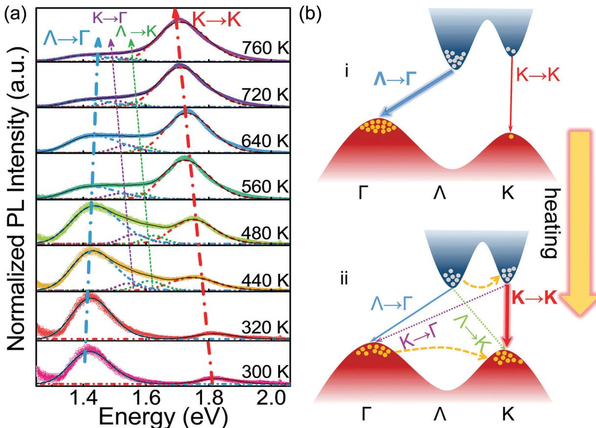
Fig. 3 (a) Multi-peak deconvolution fittings of the TD-PL spectra, showing the specific variation of each sub-peak at different temperatures. (b) Schematic diagram illustrating the excited-state carrier distribution and possible radiative transition routes at (i) room temperature and (ii) high temperature; the carrier population at the  $K$  point is effectively increased due to the heat-induced inter-valley transfer process in panel (ii).
