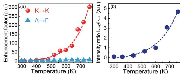
Fig. 4 (a) Enhancement factor of the  $K \rightarrow K$  direct and  $A \rightarrow \Gamma$  indirect emissions at different temperatures. (b) Temperature dependence of the integrated intensity ratio of the  $K \rightarrow K$  direct emission to the  $A \rightarrow \Gamma$  indirect emission ( $I_{K \rightarrow K}/I_{A \rightarrow \Gamma}$ ).
