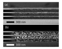
Fig. 3 Cross-sectional SEM images of a representative 6-layer BS on a silicon substrate acquired with a (a) back-scattered electron detector and (b) In-Lense detector. The MOF layers are highlighted in black, the TiO2 in white
