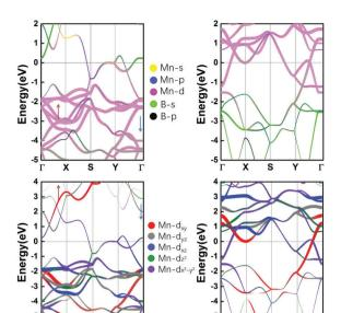
Fig. 3 Atom-projected and orbital-projected band structures of MnB sheets in spin-up and spin-down channels, and the Fermi levels are set to zero
