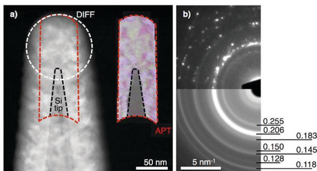
**Fig. 4** TEM of a CrMnFeCoNi film on a Si tip in state  $S_7$  (350 °C). (a) High angle annular dark field image showing the tip and the grain structure of the film ( $S_7$ , TEM) in comparison to an APT analysis from a tip from the same CPP and state ( $S_7$ ). (b) Electron diffraction acquired from the encircled region in (a) and its rotational averaging with measured interplanar distances in nm.
