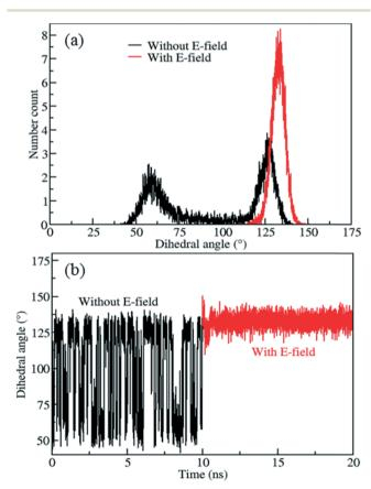
Fig. 6 a) Distribution of rotational dihedral angle of IRMOF-7-Cl ligands and b) their mean values as a function of time at 300 K with and without E-field (5 V nm<sup>-1</sup>).
