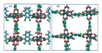
Fig. 10 Snapshots of CRO-CROp substituted IRMOF-7-Cl2 in the x-direction obtained from methane diffusion simulations (a) before and (b) after the E-field (2 V nm<sup>-1</sup>) is applied. Methane molecules are not shown for clarity.
