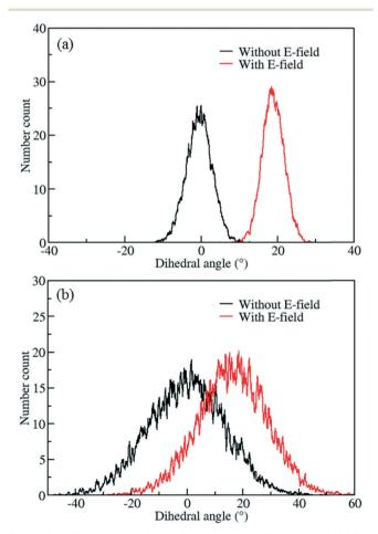
Fig. 4 Distribution of rotational dihedral angles of ligands in IRMOF-1-Cl at a) 100 K and b) 300 K with and without E-field (8 V nm<sup>-1</sup>).
