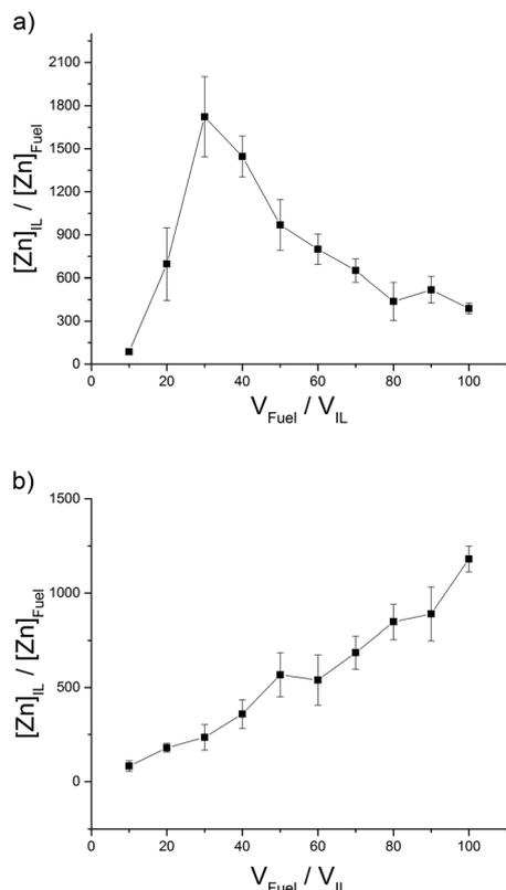
Fig. 3 ILs with intermediate distribution (I) of Zn<sup>2+</sup> into the IL phase; (a) [(CH<sub>3</sub>)<sub>2</sub>NH<sub>2</sub>][[(CH<sub>3</sub>)<sub>2</sub>NCOO]] (b) [C<sub>8</sub>C<sub>1</sub>im]Cl.
