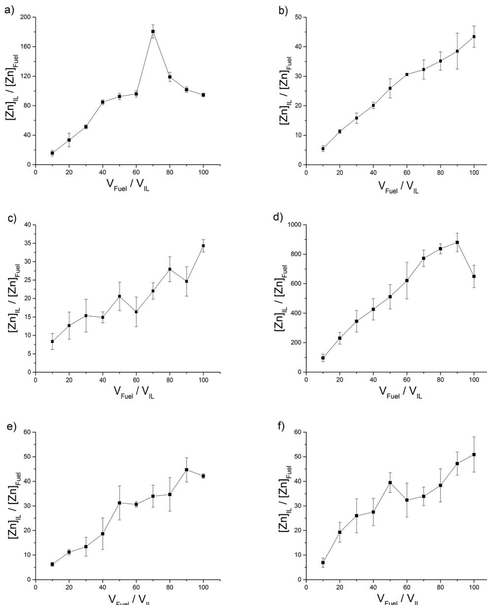
Fig. 4 ILs with a low distribution (L) of  $\text{Zn}^{2+}$  into the IL phase, (a)  $[\text{C}_4\text{C}_1\text{im}][\text{MeSO}_4]$ , (b)  $[\text{C}_4\text{C}_1\text{im}][\text{OTf}]$  (c)  $[\text{C}_4\text{C}_1\text{pyrr}][\text{OTf}]$ , (d)  $[\text{C}_8\text{C}_1\text{im}][\text{OTf}]$  and (e)  $[\text{C}_4\text{C}_1\text{im}][\text{N}(\text{Tf})_2]$  (f)  $[\text{C}_4\text{C}_1\text{pyrr}][\text{N}(\text{Tf})_2]$ .
