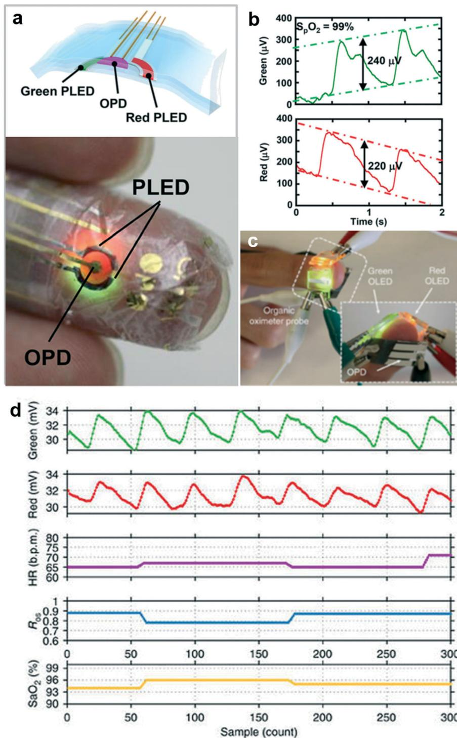
**Fig. 14** Reflectance based layout and application picture of the pulse oximeter system with concentric LED's and circular photodiode scheme (a), with resulting signal output (b). Organic transmission based oximeter (c) with resulting raw data and signal extraction (d).
