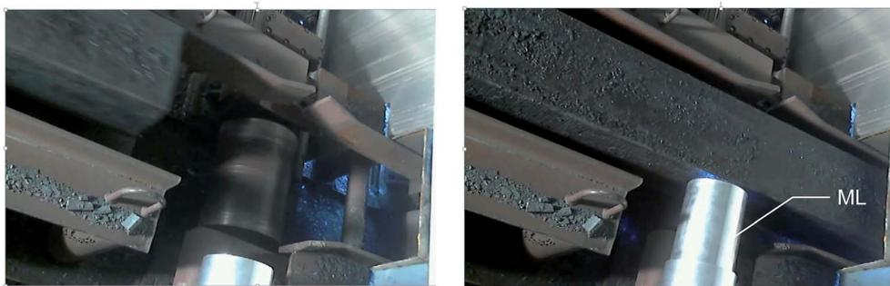
Fig. 7 Inline measurement of steel blooms, left: the bloom is transported on a roller table and arriving from the left, right: the measuring lance (ML) is approached to the side face of the bloom, laser irradiation is activated to locally ablate the scale layer and to analyse the bulk composition. Diameter of ML: 170 mm.<sup>32</sup>
