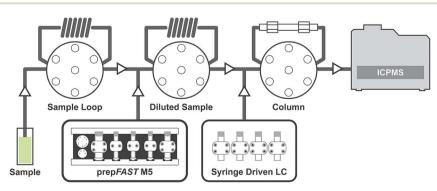
Fig. 1 Simplified flow path diagram for the prepFAST IC.
