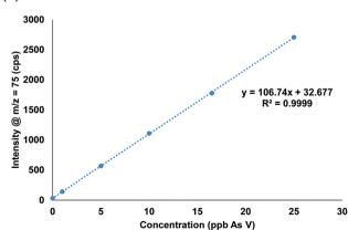
Fig. 4 (a) Chromatograms from the inline autocalibration of arsenic species, calibration standards range from 0 ppb (blank urine) up to 27 ppb. (b) Calibration curve for arsenic V.
