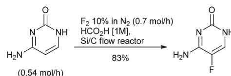
**Scheme 14** Synthesis of flucytosine using fluorine gas.
