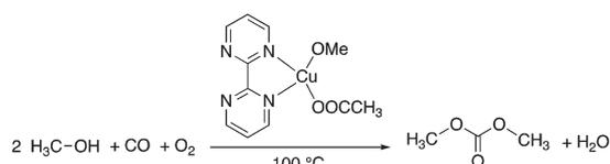
**Scheme 7** Oxidative carbonylation of methanol to dimethyl carbonate.
