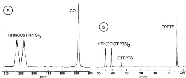
**Fig. 1**  $^{13}\text{C}$  NMR (a) and  $^{31}\text{P}$  NMR (b) spectra of  $\text{HRh}(^{13}\text{CO})(\text{TPPTS})_3$  in the presence of a 3 molar excess of TPPTS under a 200 bar pressure of  $^{13}\text{CO} : \text{H}_2 = 1 : 1$  in  $\text{D}_2\text{O}$ . Modified with permission from ref. 59. Copyright of Springer (1989).
