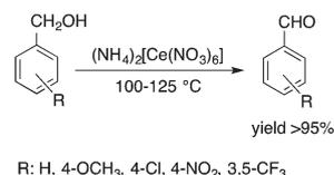
**Scheme 13** Oxidation of benzyl alcohol and its derivatives.
