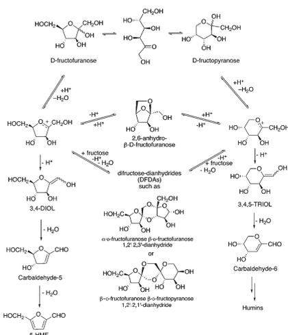
**Scheme 41** Proposed intermediates of the acid-catalyzed dehydration of D-fructose to 5-HMF *via* a cyclic pathway, adapted with permission from ref. 171. Copyright 2012 of the Royal Society of Chemistry.
