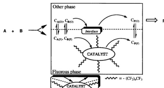
**Fig. 2** Original drawing of the fluorous biphasic concept for the catalytic conversion of substrates A and B to product P. Adapted from ref. 93. Copyright of The American Association for the Advancement of Science (1994).
