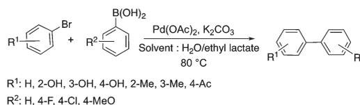
**Scheme 22** Cross-coupling reactions in a water/ethyl lactate mixture.
