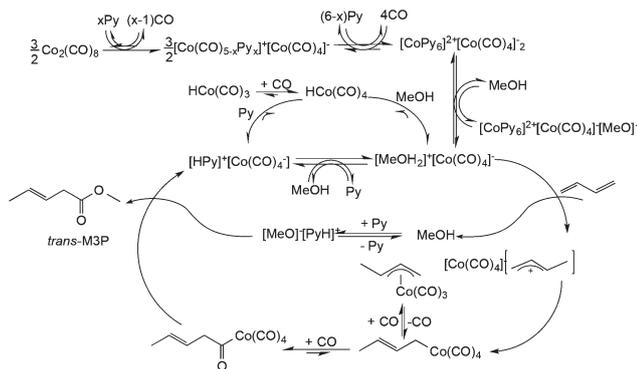
**Scheme 40** Proposed catalytic cycle of the hydromethoxycarbonylation of butadiene by pyridine-modified cobalt catalysts in methanol. Adapted with permission from ref. 170. Copyright of the American Chemical Society (2011).
