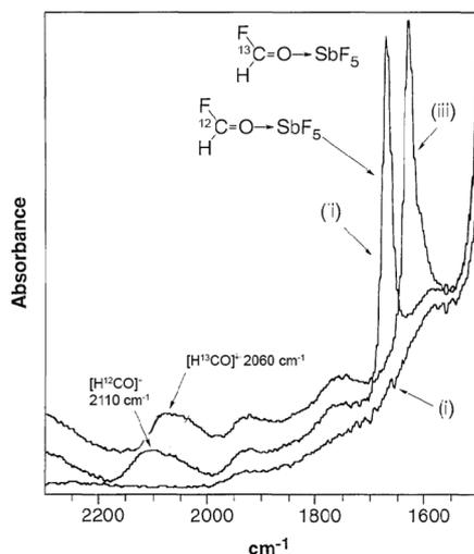
**Fig. 5** IR spectra of (i)  $\text{HF-SbF}_5$ , (ii)  $\text{HF-SbF}_5 + {}^{12}\text{CO}$ , and (iii)  $\text{HF-SbF}_5 + {}^{13}\text{CO}$ . Modified with permission from ref. 166. Copyright of The American Association for the Advancement of Science (1997).
