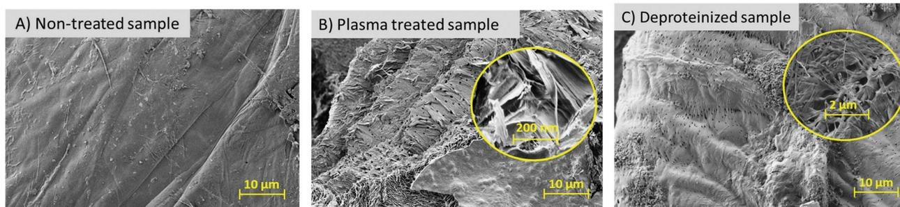
**Fig. 4** SEM images of (A) the non-treated shrimp shell, (B) the shrimp shell treated with pure  $N_2$  plasma for 6 minutes and (C) the deproteinized shrimp shell (1 M NaOH, 4 h at  $80\text{ }^\circ\text{C}$ ).
