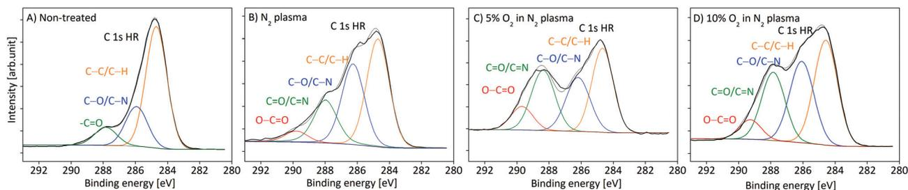
Fig. 2 XPS deconvolution of the HR C 1s spectrum for (A) the non-treated sample and the samples treated for 3 minutes with (B) pure  $\text{N}_2$  plasma, (C) 5%  $\text{O}_2$  in  $\text{N}_2$  plasma and (D) 10%  $\text{O}_2$  in  $\text{N}_2$  plasma.
