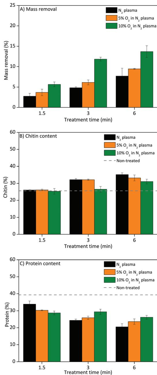
Fig. 1 Shrimp shell treatment with N<sub>2</sub> plasma, 5% O<sub>2</sub> in N<sub>2</sub> plasma and 10% O<sub>2</sub> in N<sub>2</sub> plasma for 1.5, 3 and 6 minutes. (A) Mass removed, (B) chitin content and (C) protein content. (The composition of the non-treated shrimp shell was: chitin 25.5%, protein 37.4% and mineral (ash) content 37.1%.)
