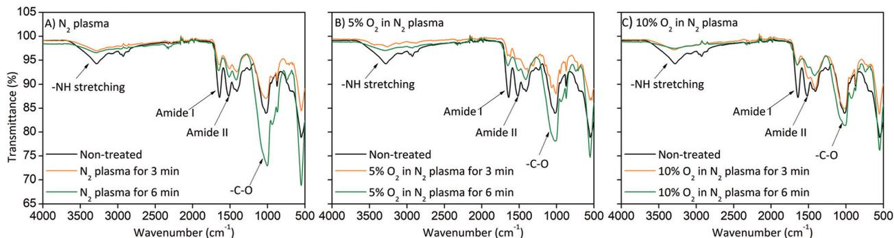
**Fig. 3** FTIR spectra of the non-treated shrimp shell and shrimp shells treated for 3 and 6 minutes with (A) pure  $N_2$  plasma, (B) 5%  $O_2$  in  $N_2$  plasma and (C) 10%  $O_2$  in  $N_2$  plasma.
