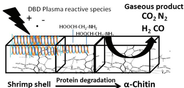
Scheme 1 Solvent-less DBD plasma-based removal of proteins from shrimp shell waste, exposing the α-chitin biopolymer and forming only gaseous products.
