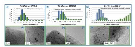
Fig. 3 Particle size distribution weighted by number (blue, from a TEM study) and by volume (green, to be used to estimate the average coordination number *N* obtained by the EXAFS first shell analysis) in three different examples of Pt NPs formed inside a Pt-functionalized UiO-67 MOF. Adapted by permission of the Royal Society of Chemistry (copyright 2017).<sup>5</sup>
