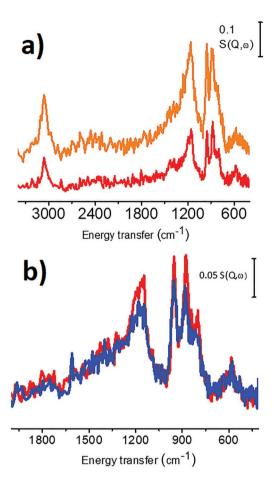
Fig. 5 Part (a) INS spectra of  $C_w$  (red spectrum) and  $C_{Chemi}$  (orange spectrum). Part (b) INS spectra of  $C_w$  (red) and of the corresponding Pd/ $C_w$  catalyst (blue). Previously unpublished figure, reporting data published in ref. 1.
