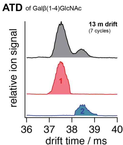
**Fig. 2** (Top) Ion mobility arrival time distribution (ATD) of the sodiated disaccharide Gal $\beta$ (1-4)GlcNAc after seven cycles SLIM mobility separation. The portions selected by electrostatic deflection of unwanted ions for further spectroscopic analysis are displayed in red (species 1) and blue (species 2), respectively.
