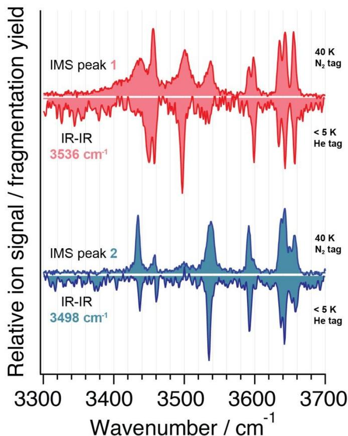
**Fig. 4** IR spectra of two conformers of Gal $\beta$ (1-4)GlcNAc acquired with the IR-IR double resonance method (downward pointing) with the pump laser fixed at 3536  $\text{cm}^{-1}$  (red) and at 3498  $\text{cm}^{-1}$  (blue), respectively. The spectra of the ion-mobility separated species 1 and 2 (upward pointing) are displayed for comparison in red and blue, respectively.
