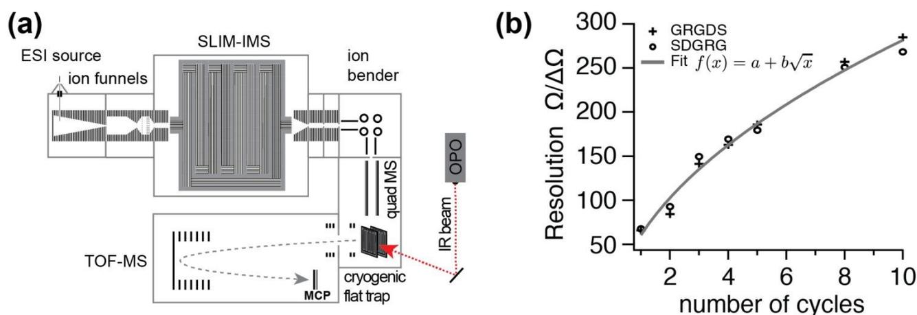
**Fig. 1** (a) Schematic overview of the instrument combining ultra-high resolution SLIM IMS techniques with messenger-tagging IR spectroscopy. (b) IMS resolution of the new instrument as a function of SLIM cycles (IMS path length) determined by monitoring the peak widths and positions of two isomeric MS standard peptides GRGDS and SDGRG in their doubly protonated form.
