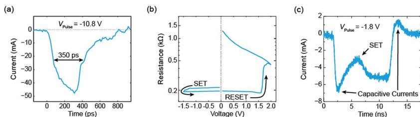
Fig. 5 Selected measurements from ref. 17. (a) The current response of an electrical voltage pulse with an amplitude of  $-10.8 \text{ V}$ . Its FWHM amounts to 350 ps. The subsequent  $I$ - $V$  sweep is shown in (b). As it starts in the LRS, the ReRAM device must have set during the application of the 350 ps pulse. In (c) the current response of a 10 ns voltage pulse with an amplitude of  $-1.8 \text{ V}$  is shown. It is possible to resolve the set event after about 5 ns.
