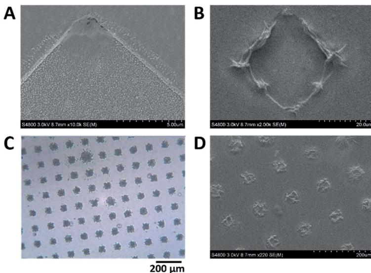
Fig. 6 Scanning electron microscopy (SEM) images of the MNEE array after (A) 5 seconds and (B) 10 seconds growth at  $50 \mu\text{A}$ . A close up of the electrode in (A) can be found in Fig. S3† showing that gel is growing across the entire electrode but enhanced growth is clearly occurring in the corners. (C) and (D) are light microscopy and SEM images of a collapsed (dehydrated) hydrogel, respectively, after 20 s, which show that hydrogel has completely filled each cavity in the array.
