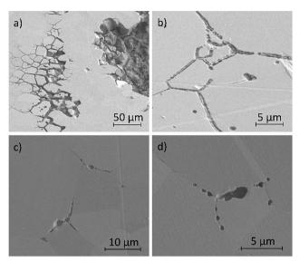
Fig. 11 A series of secondary electron images of different areas of the corroded sensitised AISI 304 stainless steel surface showing localised corrosion. Images (a) and (b) were taken at a tilt of  $52^{\circ}$ , and (c) and (d) were taken at a tilt of  $0^{\circ}$ .
