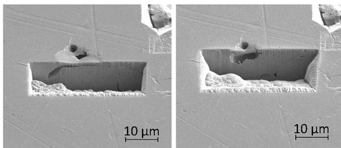
Fig. 13 Secondary electron images taken as a part of a series of 2–5  $\mu\text{m}$  thick slices into a region of the material surrounding an intragranular pit using FIB, taken at a tilt of  $52^\circ$ .
