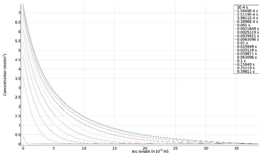
Fig. 10 A line plot produced in COMSOL showing the concentration of  $\text{Fe}^{2+}$  ions along a line normal to the metal surface, starting from the centre of the pit and extending out to the bulk solution, for different time steps.
