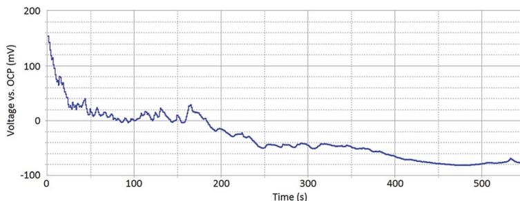
Fig. 3 A galvanostatic scan of a sensitised AISI 304 stainless steel sample within 1% aqueous NaCl taken at 0.05 mA, for a sample surface area of 0.13 cm<sup>2</sup>.
