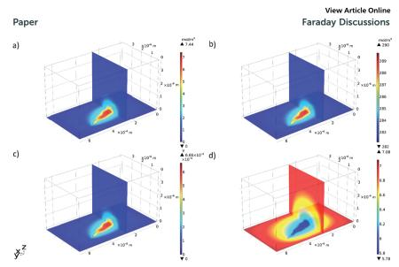
Fig. 9 3D multi-slice plots produced in COMSOL showing the final (at a time of 0.5 s): (a) concentration of Fe<sup>2+</sup> ions, (b) concentration of Cl<sup>-</sup> ions, (c) electrolyte potential, and (d) pH.
