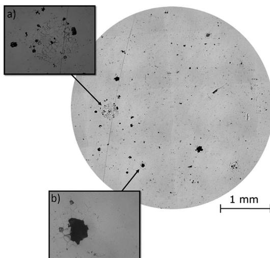
Fig. 4 A mosaic photo of the sensitised AISI 304 stainless steel sample surface post-corrosion, taken with a Leica optical microscope with a 5 $\times$  optical objective, with additional photos of specific areas of interest taken with an Olympus BH2-UMA optical microscope at magnifications of (a) 20 $\times$  and (b) 50 $\times$ .
