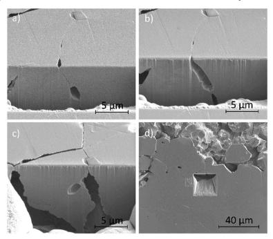
Fig. 12 Secondary electron images taken as a part of a series of  $2-5~\mu m$  thick slices into a region of the material surrounding an intergranular pit using FIB. Images (a)–(c) were taken at a tilt of  $52^{\circ}$ , and (d) was taken at a tilt of  $0^{\circ}$ .
