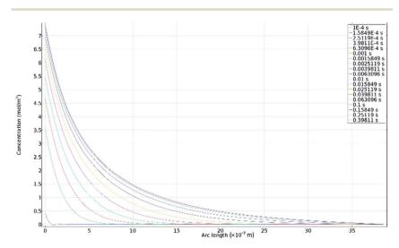
Fig. 10 A line plot produced in COMSOL showing the concentration of  $Fe^{2+}$  ions along a line normal to the metal surface, starting from the centre of the pit and extending out to the bulk solution, for different time steps.
