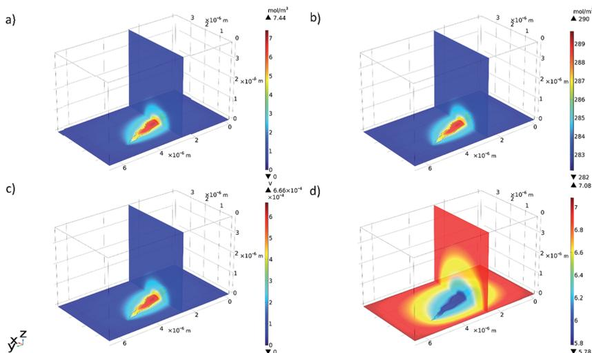
Fig. 9 3D multi-slice plots produced in COMSOL showing the final (at a time of 0.5 s): (a) concentration of  $\text{Fe}^{2+}$  ions, (b) concentration of  $\text{Cl}^-$  ions, (c) electrolyte potential, and (d) pH.
