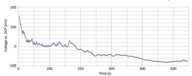
Fig. 3 A galvanostatic scan of a sensitised AISI 304 stainless steel sample within 1% aqueous NaCl taken at 0.05 mA, for a sample surface area of 0.13 cm<sup>2</sup>.
