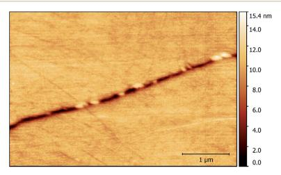
Fig. 5 A topographic map showing inclusions along a GB in sensitised AISI 304 stainless steel within 1% aqueous NaCl.
