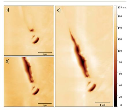
Fig. 7 Topographic maps showing a GB in sensitised AISI 304 stainless steel within 1% aqueous NaCl: (a) before formation of intergranular pit, (b) after formation of intergranular pit, and (c) the full intergranular pit formed.
