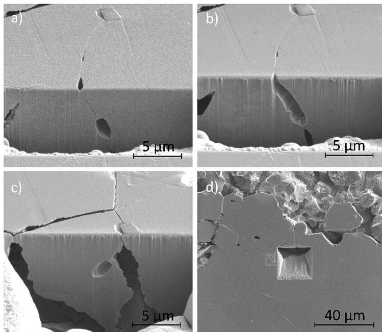
Fig. 12 Secondary electron images taken as a part of a series of 2–5  $\mu\text{m}$  thick slices into a region of the material surrounding an intergranular pit using FIB. Images (a)–(c) were taken at a tilt of  $52^\circ$ , and (d) was taken at a tilt of  $0^\circ$ .
