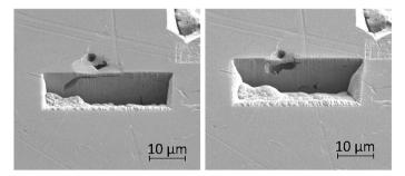
Fig. 13 Secondary electron images taken as a part of a series of  $2-5 \mu m$  thick slices into a region of the material surrounding an intragranular pit using FIB, taken at a tilt of  $52^{\circ}$ .
