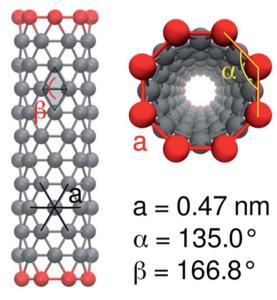
Fig. 2 MARTINI model of a CNT with  $12 \times 8$  nonpolar CNP beads and polar end groups, with angles and bond lengths indicated.
