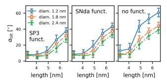
Fig. 9 Tilting angle of the CNTs in POPC lipid membranes. Results are shown for coarsegrained simulations as a function of the CNT length for three different CNT diameters. The polarity of the rim decreases from left to right, with functionalization indicated in the figure. Vertical bars denote the standard deviation.
