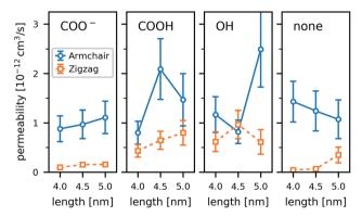
Fig. 11 Water permeability  $p_{\rm f}$  calculated from the MSD of the net permeation n(t) in equilibrium atomistic simulations of single CNT porins in a POPC lipid membrane. Results are shown for two chiralities (armchair, zigzag), three CNT lengths (4.0 nm, 4.5 nm, and 5.0 nm), and rims with four different functionalizations (COO $^-$ , COOH, OH, none). Vertical bars denote the standard error estimated from block averaging using 12 blocks.
