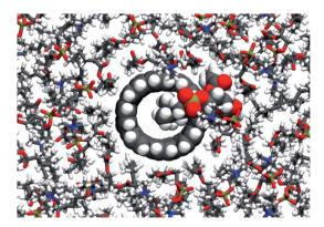
**Fig. 6** Head group of a POPC molecule blocking the pore of a non-functionalized armchair CNT of 4 nm length. In this view down onto the membrane, atoms of the CNT and the pore-blocking lipid are shown as spheres and the bonds of surrounding lipids as sticks.
