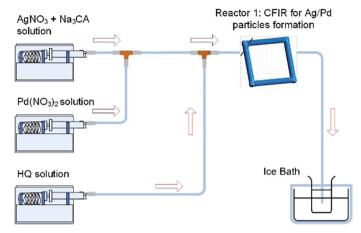
Fig. 11 Simultaneous reduction of Aq(NO<sub>3</sub>) and Pd(NO<sub>3</sub>)<sub>2</sub> with HQ in a CFI microreactor.
