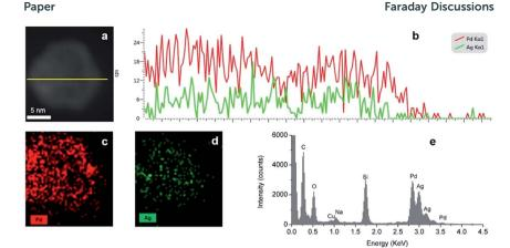
Fig. 7 (a and b) EDS line scan of the Ag-Pd hollow NPs, (c and d) EDS elemental mapping of Ag-Pd hollow NPs, (e) EDS spectra of the Ag-Pd hollow NPs after Reactor 3 using  $Pd(NO_3)_2$  as precursor.
