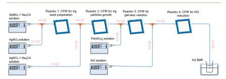
Fig. 8 Synthesis of hollow Ag–Pd bimetallic nanoparticles using CFI reactors connected in series for the separation of the galvanic displacement and co-reduction steps.
