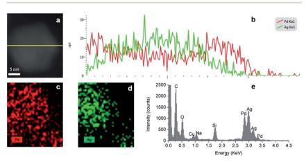
Fig. 14 (a and b) EDS line scan, (c and d) EDS elemental mapping and (e) EDS spectra of Ag-Pd alloy NPs synthesised by simultaneous reduction of  $Ag(NO_3)$  and  $Pd(NO_3)_2$  with HQ.
