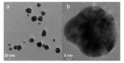
Fig. 13 (a) TEM and (b) HRTEM image for Ag-Pd alloy NPs synthesized by simultaneous reduction of  $Aq(NO_3)$  and  $Pd(NO_3)_2$  with HQ.
