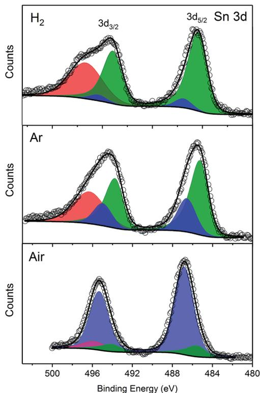
Fig. 3 Sn 3d XPS spectra of samples synthesized under H<sub>2</sub>/N<sub>2</sub>, Ar or air. Peak deconvolution shown corresponding to Sn<sup>0</sup> (green), Sn<sup>IV</sup> (blue), and metallic Sn 3d<sub>3/2</sub> (red).
