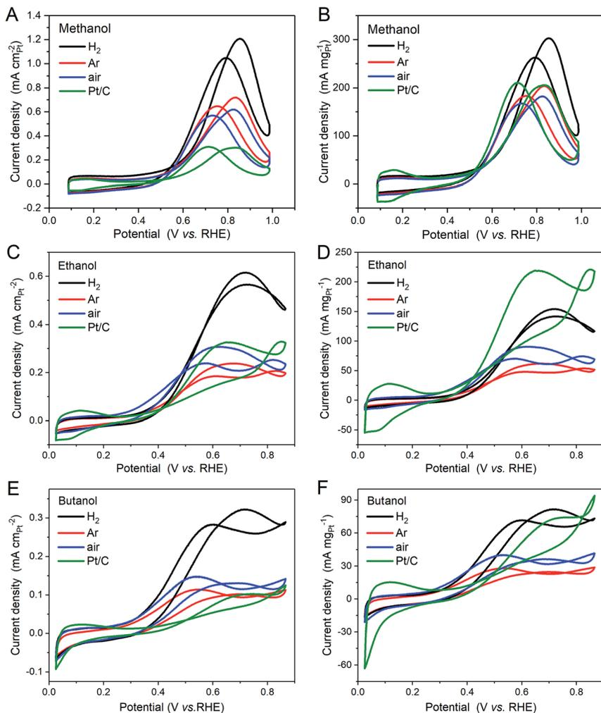
Fig. 7 Cyclic voltammograms illustrating the specific activities (A, C and E) and mass activities (B, D and F) of the heat treated  $\text{Pt}_3\text{Sn}$  catalysts and the commercial Pt/C reference catalyst in  $0.1 \text{ mol dm}^{-3} \text{ H}_2\text{SO}_4$  and  $0.1 \text{ mol dm}^{-3}$  (A and B) methanol, (C and D) ethanol, and (E and F) 1-butanol at  $25^\circ \text{C}$  with a scan rate of  $50 \text{ mV s}^{-1}$ .
