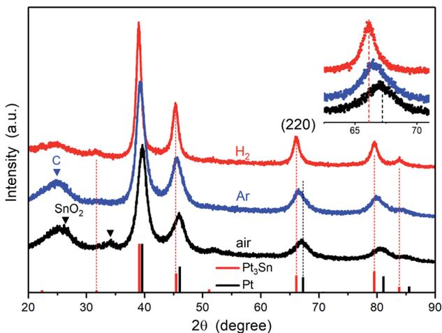
Fig. 2 XRD patterns of Pt<sub>3</sub>Sn nanoparticles annealed under H<sub>2</sub>, Ar and air. The inset shows the magnified region of the (220) peak. The standard patterns of Pt<sub>3</sub>Sn (35-1360) and Pt (04-0802) were obtained from the JCPDS database.
