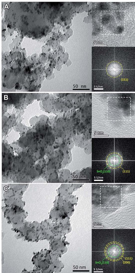
Fig. 1 TEM images of  $\text{Pt}_3\text{Sn}$  nanoparticles annealed under (A)  $\text{H}_2$ , (B) Ar and (C) air. The upper insets are the corresponding HRTEM images and the bottom insets are the fast-Fourier transform patterns on the selected area (white dashed square) in the corresponding HRTEM images. The dashed rings are drawn to connect bright spots at the same distance to the centre and represent the lattice fringes of the selected areas.
