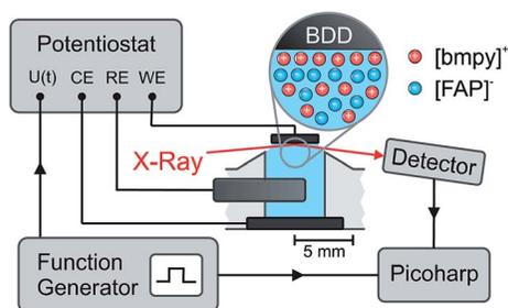
Fig. 2 The potential  $U$  between the working electrode (WE) and the quasi reference electrode (RE) is controlled by a potentiostat in a standard 3-electrode configuration with a counter electrode (CE). For XRR measurements with sub-millisecond time resolution, a periodic square wave potential  $U(t)$  was applied by an external function generator. A Picoharp device assigned a time stamp to each photon counting event recorded by the detector and the rising edge of the potential steps.
