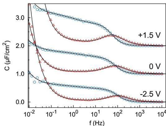
Fig. 3 Imaginary part (red triangles) and real part (blue circles) of the complex differential capacitance at the potentials +1.5 V (top), 0 V (middle) and  $-2.5$  V (bottom). Lines are fits to the Cole–Cole expression (eqn (9)). Curves are vertically shifted by 1 unit for clarity.
