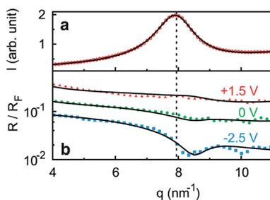
Fig. 5 (a) Bulk X-ray scattering pattern (symbols) of  $[\text{bmpy}]^+[\text{FAP}]^-$ . The dashed vertical line indicates the peak position (b) measured (symbols) XRR curves  $R(q)$  normalized by the Fresnel reflectivity  $R_F(q)$  of an ideally flat and abrupt IL/BDD interface. Lines show simultaneous fits of all three curves to the modified distorted crystal model. The  $0 \text{ V}$  and  $-2.5 \text{ V}$  curves are shifted for clarity.
