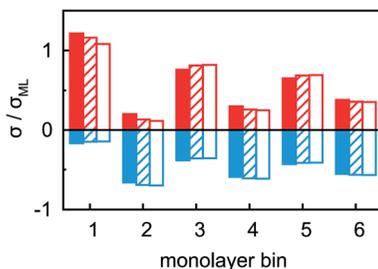
Fig. 7 Anion (blue) and cation (red) charges  $\sigma$  in the  $n$ -th IL layer, counted from the BDD interface, at potentials  $-2.5$  V (solid),  $0$  V (hatched) and  $+1.5$  V (empty). Charges are normalized to the equivalent of a full monolayer  $\sigma_{ML} = 19 \mu\text{C cm}^{-2}$ .
