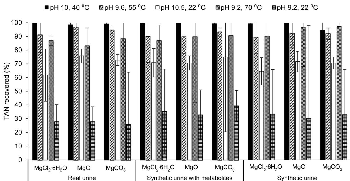
**Fig. 1** Effect of ammonia stripping–acid absorption conditions, Mg sources, and urine solution on TAN recovery *via* ammonia stripping–acid absorption after 3 h of operation. Urine composition and struvite precipitation conditions reported on x-axis labels. Ammonia stripping–acid absorption conditions reported in legend. All measured data are average values of triplicate samples with error bars showing one standard deviation.
