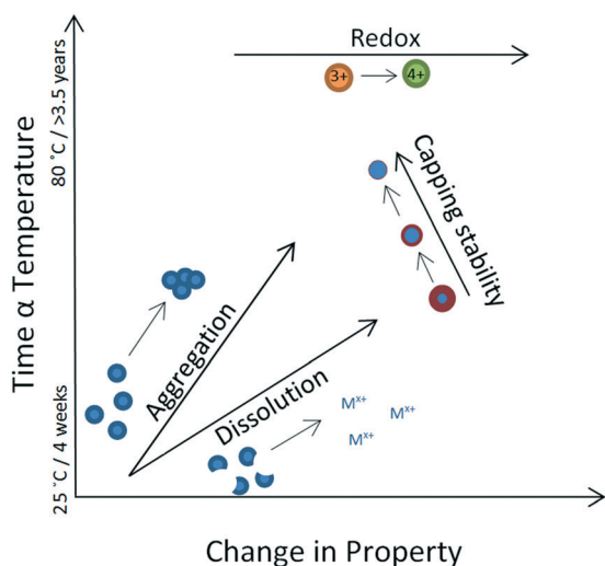
Fig. 6 Schematic depicting change in NM properties as a function of temperature, as a proxy for time for 40k PVP capped ceria as an example. The arrows show the direction of change for each property, specifically: from a lower to higher oxidation state, from a disaggregated to aggregated state, from larger to smaller individual particles due to dissolution and from the capped to uncapped state. Though not always the case for all samples, in this case the transformations occur in a linear fashion and the rate varies (as shown by the gradient in the slope of individual arrows).
