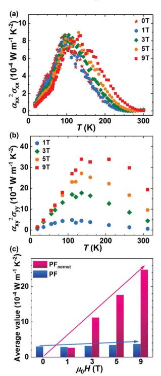
Fig. 2 The power factor PF  $\alpha_{xx}^2 \sigma_{xx}$  (a), Nernst power factor PF<sub>Nernst</sub>  $\alpha_{xy}^2 \sigma_{yy}$ (b) and average values of PF and  $PF_{Nernst}$  over the investigated temperature range (c) for polycrystalline NbP under different magnetic fields.
