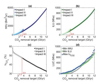
Fig. 8 Minimal water use (a), minimal land use (b), maximal CO<sub>2</sub> efficiency (c) under impact scenario I (DEC on MAL), II (DEC on MAL and AR) and III (all land types, all crops) and land use change in impact scenario III under the three optimisation scenario (d).
