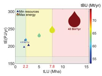
Fig. 10 BECCS total electricity generated under different land constraints, in the energy maximisation scenario (droplets), and the water, land and  $\rm CO_2$  efficiency minimisation and maximisation scenarios (triangles). Water use is represented by the colour scale, and biomass use, by the markers' size. Even when land use is constrained to a "safe" value (green zone), the UK electricity generation objective consistent with a 50  $\rm Mt_{\rm CO_2}$  per year target is met.
