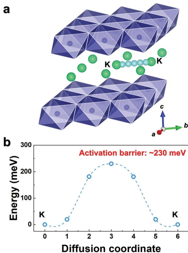
Fig. 7 (a) K–K diffusion pathways into the  $K_{0.69}$ CrO<sub>2</sub> structure. (b) Activation barrier energy for K<sup>+</sup> diffusion in  $K_{0.69}$ CrO<sub>2</sub> obtained using NEB calculations.
