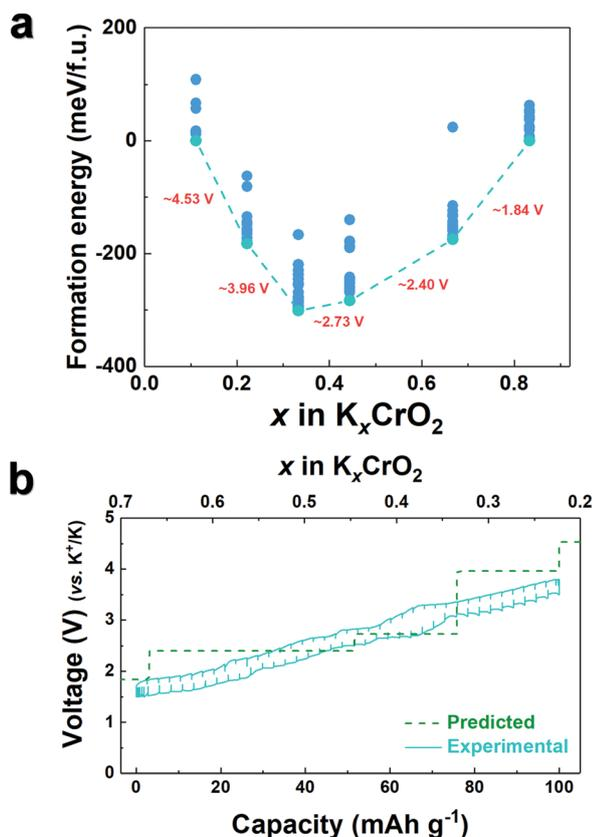
Fig. 3 (a) Formation energy of  $\text{K}_x\text{CrO}_2$  ( $0.11 \leq x \leq 0.83$ ) and (b) comparison of experimentally measured GITT charge-discharge curves and predicted voltage curves obtained using first-principles calculations.
