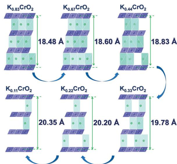
Fig. 4 Predicted structural changes of  $\text{K}_x\text{CrO}_2$  as a function of the K content ( $0.11 \leq x \leq 0.83$ ) using first-principles calculations.
