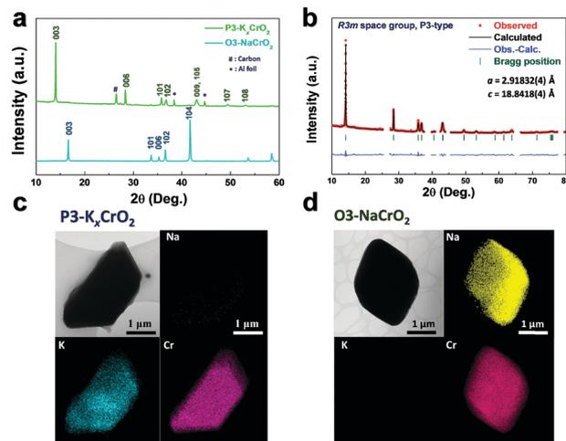
Fig. 2 (a) Comparison of the XRD patterns for the P3-K<sub>x</sub>CrO<sub>2</sub> electrode and O3-NaCrO<sub>2</sub> powder. (b) Profile-matched XRD patterns of P3-K<sub>x</sub>CrO<sub>2</sub> using Rietveld refinement ( $R_p = \sim 1.65\%$ ,  $R_1 = \sim 1.28\%$ ,  $R_f = \sim 2.07\%$ , and  $\chi^2 = \sim 7.43\%$ ). TEM images and the corresponding EDX mapping of (c) P3-K<sub>x</sub>CrO<sub>2</sub> and (d) O3-NaCrO<sub>2</sub>.
