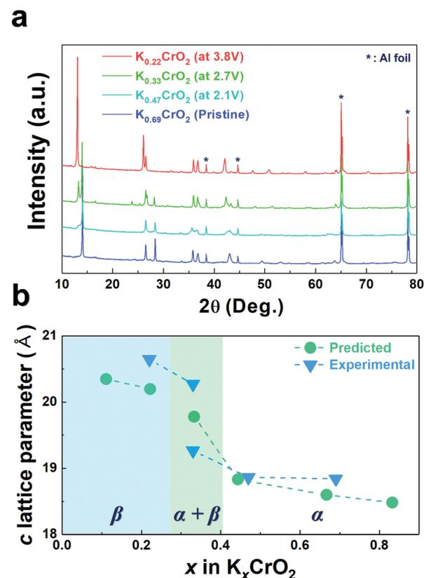
Fig. 5 (a) *Ex situ* XRD patterns of the  $\text{K}_x\text{CrO}_2$  samples with various K contents and (b) comparison of the c lattice parameters of  $\text{K}_x\text{CrO}_2$  predicted based on first-principles calculations and experimental results.
