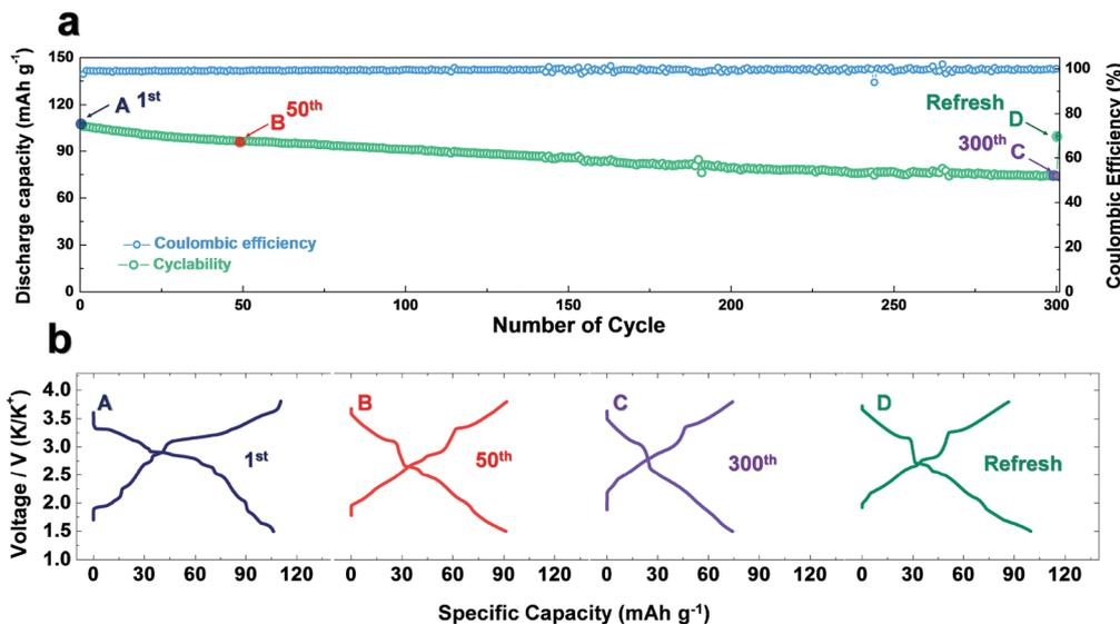
Fig. 1 Electrochemical ion-exchange process: (a) multiple cycling process of K metal|0.5 M KPF<sub>6</sub> in a EC : DEC = 1 : 1 (v/v)|NaCrO<sub>2</sub> cell at 1C rate (100 mA g<sup>-1</sup>) and (b) corresponding charge–discharge voltage curves at the 1st, 50th, 300th cycle and the refreshed cell at 0.1C rate (10 mA g<sup>-1</sup>).
