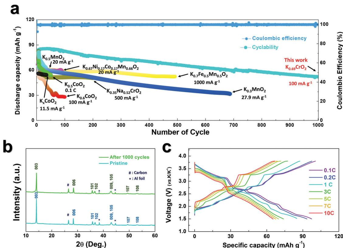
Fig. 6 (a) Cyclability of  $\text{K}_{0.69}\text{CrO}_2$  over 1000 cycles at 1C rate and comparison of specific capacity vs. cycle number for the layered oxide cathode for this work and previous studies. (b) *Ex situ* XRD patterns of the  $\text{K}_{0.69}\text{CrO}_2$  electrode for the pristine sample and after 1000 cycles. (c) Power capability of  $\text{K}_{0.69}\text{CrO}_2$  at various current rates (0.1C, 0.2C, 1C, 3C, 5C, 7C, and 10C).
