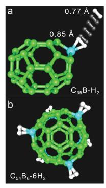
Fig. 12 Structural model illustrating inclusion of one (a) or six (b) boron atoms in a fullerene and their interaction with molecular H2; green, blue, and white spheres represent C, B, and H atoms, respectively. Reprinted Fig. 1 and 4 (adapted) with permission from Y.-H. Kim, Y. Zhao, A. Williamson, M. J. Heben and S. B. Zhang, Phys. Rev. Lett., 2006, 96, 016102. Copyright 2016 by the American Physical Society.
