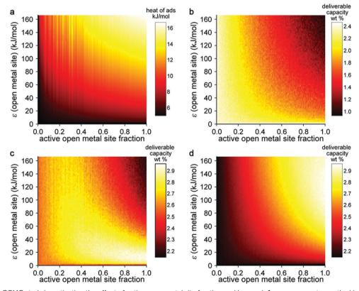
Fig. 5 Results of a GCMC study investigating the effect of active open metal site fraction and Lennard-Jones ε parameter on the H<sub>2</sub> capacity of a model system based on the Mg<sub>2</sub>(dobdc) structure type. (a) Heat of adsorption for H<sub>2</sub> at low loading; usable capacity at (b) 77 K; (c) 180 K; and (d) 243 K given a pressure swing between 100 and 5 bar
