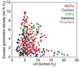
Fig. 4 Excess gravimetric H<sub>2</sub> uptake versus enthalpy of H<sub>2</sub> adsorption for various classes of hydrogen storage materials. The adsorption enthalpy values were taken from ref. 26 and 30-33 and are reported at cryogenic conditions, typically between 77 and 87 K.
