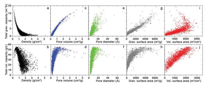
Fig. 3 Total gravimetric (top) and volumetric (bottom) capacities as a function of various crystallographic properties for 5309 MOFs extracted from the UM and CoRE databases. <sup>13,16</sup> Capacities were calculated at 77 K and 100 bar using Grand Canonical Monte Carlo (GCMC) simulations with the pseudo-Feynman–Hibbs interatomic potential. <sup>17–19</sup>
