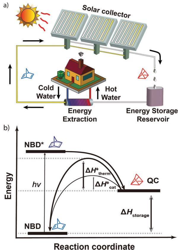
Fig. 1 (a) Operating set up based on the MOST concept. (b) Illustration of MOST molecules.  $\Delta H_{\text{therm}}^{\ddagger}$  and  $\Delta H_{\text{cat}}^{\ddagger}$  represent the activation enthalpy for QC → NBD by heat and a catalyst, respectively.  $\Delta H_{\text{storage}}$  corresponds to the energy storage enthalpy.
