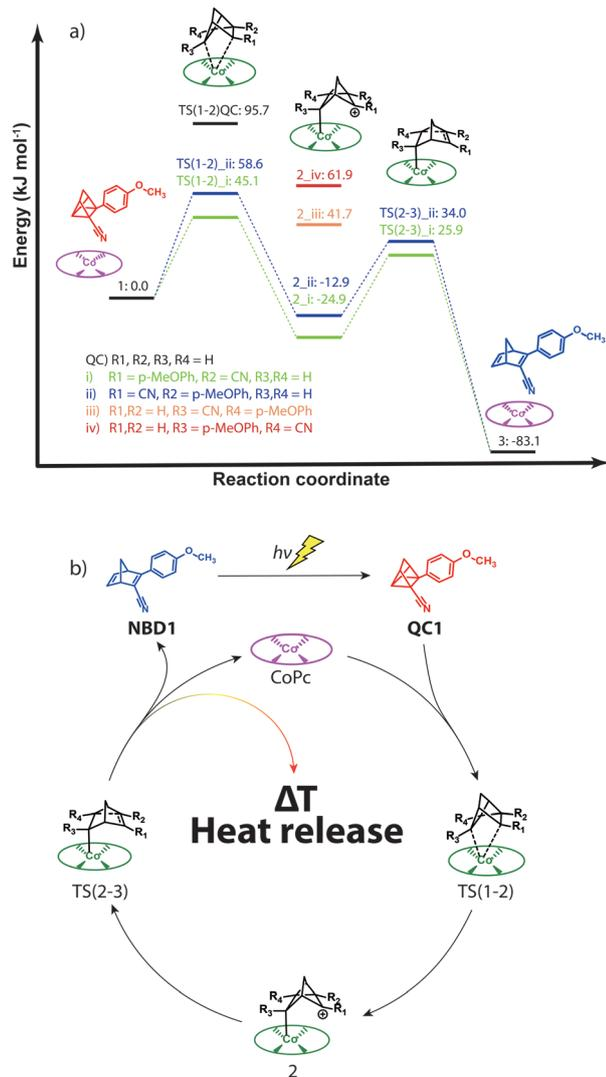
Fig. 4 (a) Critical points along the potential energy surface for the catalytic conversion of **QC1** to **NBD1** using CoPc (free energies in  $\text{kJ mol}^{-1}$  computed in toluene with respect to a 10 Å separation of CoPc and **QC1**). The color coding represents molecular structures or orientations. (b) Catalytic cycle for the back-reaction.
