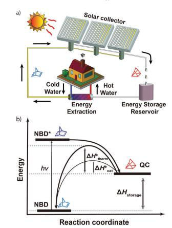
Fig. 1 (a) Operating set up based on the MOST concept. (b) Illustration of MOST molecules.  $\Delta H_{
