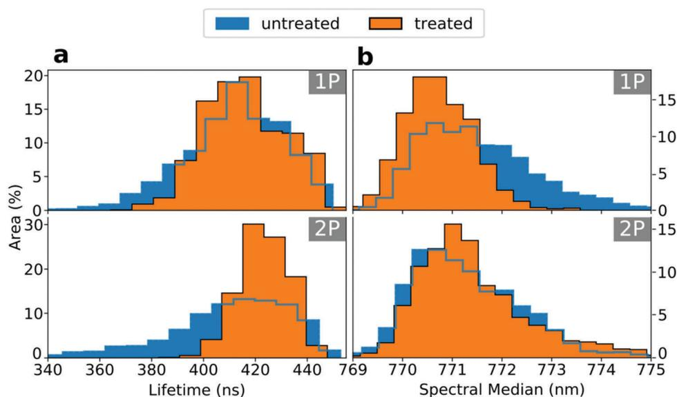
Fig. 3 Comparison between (a) PL lifetime and (b) PL spectral median distributions in the untreated (blue) and treated (orange) films, extracted from the 2D maps in Fig. 2 and Fig. S8 (ESI<sup>†</sup>) using one-photon (1P) and two-photon (2P) excitation.
