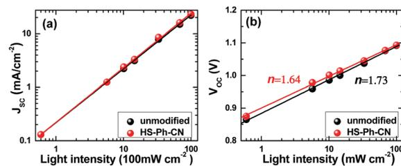
Fig. 5 Dependence of the (a)  $J_{\text{SC}}$  and (b)  $V_{\text{OC}}$  of unmodified (black) and HS-Ph-CN-treated (red)  $\text{Cs}_{0.05}\text{FA}_{0.79}\text{MA}_{0.16}\text{PbI}_{2.49}\text{Br}_{0.51}$ -based solar cells (aperture  $1.00 \text{ cm}^2$ ) on the light intensity. Lines show linear fits to the experimental data.
