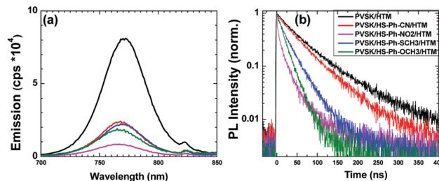
Fig. 3 Effects of benzenethiols on the photoluminescence properties of the Cs<sub>0.05</sub>FA<sub>0.79</sub>MA<sub>0.16</sub>PbI<sub>2.49</sub>Br<sub>0.51</sub>|spiro-OMeTAD system: (a) steady-state PL spectra, (b) time-resolved PL decay curves. The perovskite layer was either unmodified, or treated with HS-Ph-CN, HS-Ph-NO<sub>2</sub>, HS-Ph-SCH<sub>3</sub>, or HS-Ph-OCH<sub>3</sub>. The excitation wavelength was 465.8 nm in all experiments.
