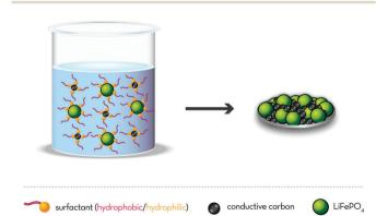
Fig. 4 Schematic illustration of the working principle of surfactants in aqueous electrode slurries, ensuring the homogenous dispersion of the hydrophobic carbon-coated LFP active material and carbon black particles (left panel) and, thus, allowing for the realization of a percolating network of the conductive agent throughout the electrode coating layer (right panel).
