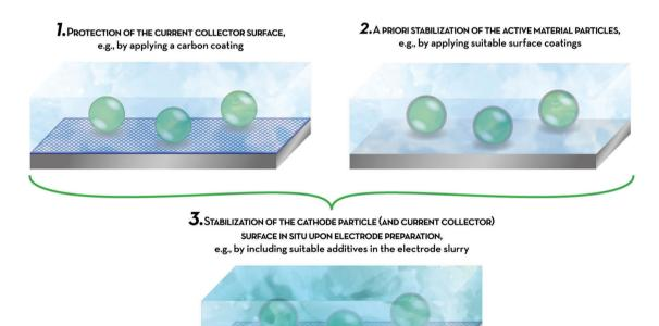
Fig. 6 (a) General challenges for the aqueous electrode processing of water-sensitive electrode materials like NCM, LR-NCM, or LNMO and (b) potential strategies to overcome these issues, including (1) the protection of the current collector surface, (2) the *a priori* stabilization of the active material particle surface, and (3) the stabilization and protection of potentially both surfaces *in situ* upon electrode preparation.
