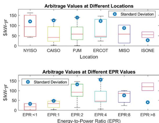
Fig. 4 Arbitrage value differentiated by location and EPR.
