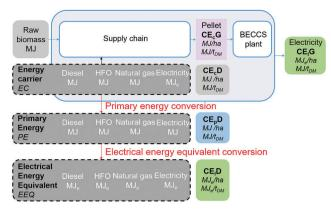
Fig. 2 Overview of the BECCS dynamic energy model. Net electricity balance, electricity return on investment and electricity pay-back time are calculated based on these metrics.
