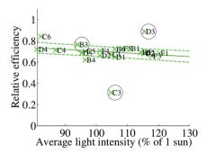
Fig. 6 Illumination level is acting as a nuisance factor of the efficiency of dye solar cells after 700 hours of aging under illumination<sup>22</sup> because the post-aging efficiencies form a line with negative slope with respect to the illumination intensity (measured separately for each cell). A reprinted derivative from ref. 22 under CC-BY license.
