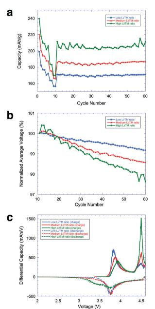
Fig. 1 A comparison of electrochemical data for LMR NMC with low, medium, and high Li/TM ratios: (a) specific capacity in half cell coin cells over various discharge rates from C/10 up to 2C, then 50 subsequent cycles at a rate of C/3. The first charge was to 4.6 V, then all following cycles were between 2.0-4.5 V vs. Li/Li<sup>+</sup>. (b) Normalized average voltage over the 50 cycles in the half cells, (c) differential capacity plot for the first cycle in the half cells
