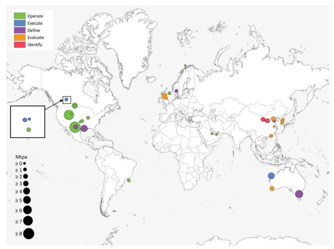
Fig. 3 Commercial-scale integrated CCS projects around the world. Circle size is proportional to the CO<sub>2</sub> capture capacity of the project and the colour indicates the lifecycle of the project. Data from the Global CCS Institute.<sup>4</sup>
