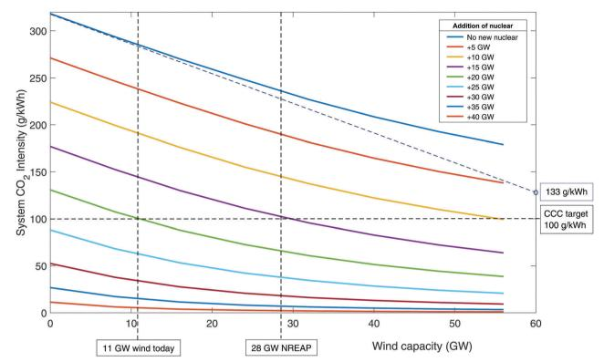
Fig. 4 The CO<sub>2</sub> emissions in 2030 as a function of wind and nuclear build when unabated CCGT is used as flexible back-up.
