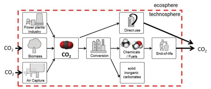
Fig. 22 Life-cycle of carbon dioxide re-use with main classes of CO<sub>2</sub> sources and utilisation pathways. The dashed box separates the technosphere from the ecosphere.
