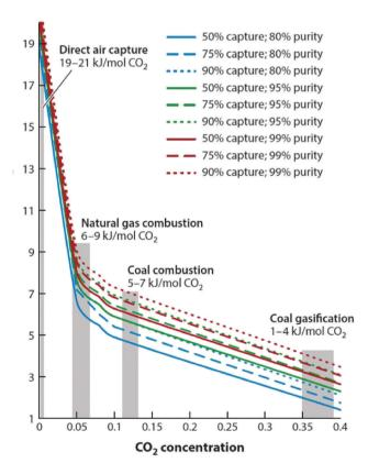
Fig. 27 Minimum work required for CO<sub>2</sub> capture based upon initial CO<sub>2</sub> concentration, capture rate, and final CO<sub>2</sub> purity. 308
