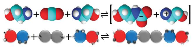
Fig. 13 SAFT physical model of  $CO_2$  chemisorption in aqueous MEA solution: the amine groups are depicted in dark blue, the hydroxyl groups in red, and  $CO_2$  in grey; the sites labelled "e" are the hydrogen-bond acceptor electron-lone pairs of the electronegative atoms, the sites labelled "H" are the donor hydrogen sites, and the sites labelled "a" are the sites mediating the reactions with  $CO_2$ .
