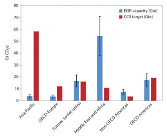
Fig. 20 Global CO<sub>2</sub>-EOR capacity compared with CO<sub>2</sub> mitigation targets. Figure reproduced from Mac Dowell et al. 967 Data from Dooley et al., 974 IEA, 975 and CIA. 976 The error bars indicate an average calculated variance of 30%. The actual reported variance is in the range of 25-35%.
