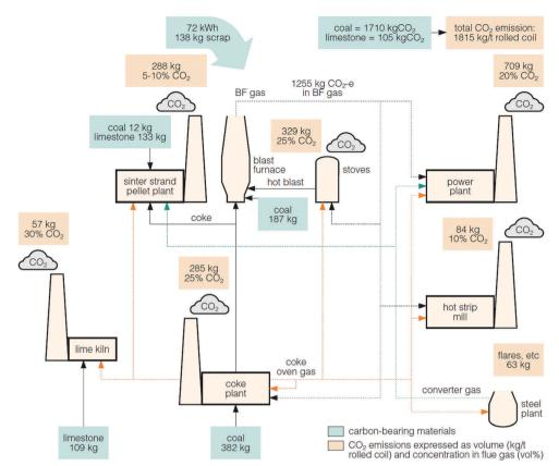
Fig. 8 A typical steel mill and the  $CO_2$  emissions, which vary in concentration. <sup>117,118</sup>
