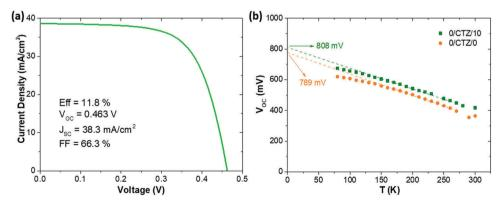
Fig. 7 (a) J-V curve corresponding to the best solar cell obtained in this work. (b)  $V_{OC}$  vs. T plot of a reference sample without Ge and a sample with 10 nm of Ge deposited on top of the CTZ precursors
