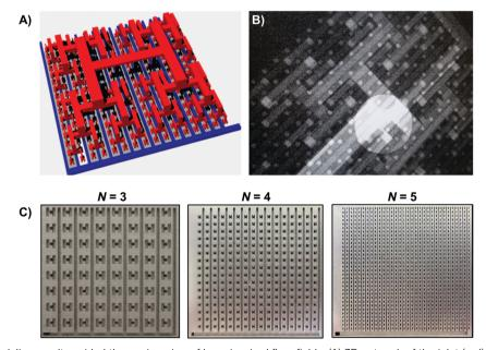
Fig. 2 The promising modeling results guided the engineering of lung-inspired flow fields: (A) 3D network of the inlet (red) and outlet (blue) branches used in these flow fields; (B) X-ray radiography is employed to inspect the flow fields for structural defects and (C) the engineered flow fields with different numbers of generations, N.
