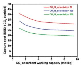
Fig. 2 Relationship between the CO<sub>2</sub> capture cost and CO<sub>2</sub> selectivity/ working capacity of solid adsorbents.<sup>8</sup> Figure reproduced with permission
