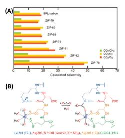
Fig. 3 (A) CO<sub>2</sub>/CH<sub>4</sub>, CO<sub>2</sub>/N<sub>2</sub>, and CO<sub>2</sub>/O<sub>2</sub> selectivities of different zeolitic imidazole frameworks (ZIFs) showing that the CO<sub>2</sub>/N<sub>2</sub> and CO<sub>2</sub>/O<sub>2</sub> selectivities follow the same trends. 30 (B) CO<sub>2</sub> capture in the active site of rubisco.<sup>40</sup> (A) Reproduced with permission from ref. 30. Copyright (2009) American Chemical Society.
