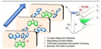
**Scheme 1** | Diagram of molecular structural engineering and the impact of enhanced-planarity and conjugation on intersystem crossing for achieving efficient organic RTP within a donor-acceptor-donor ternary  $\pi$ -conjugated framework.
