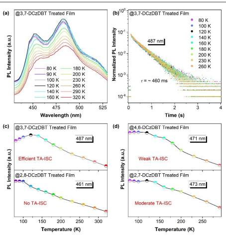
Figure 4 | (a) Phosphorescence spectra and (b) time-resolved phosphorescent decay curves at different temperatures of treated PVA films with doped 3,7-DCzDBT. The emission intensity of maximum emission peaks at different temperatures of (c) 3,7-DCzDBT and 2,8-DCzDBT, and (d) 4,6-DCzDBT and 2,7-DCzDBT.
