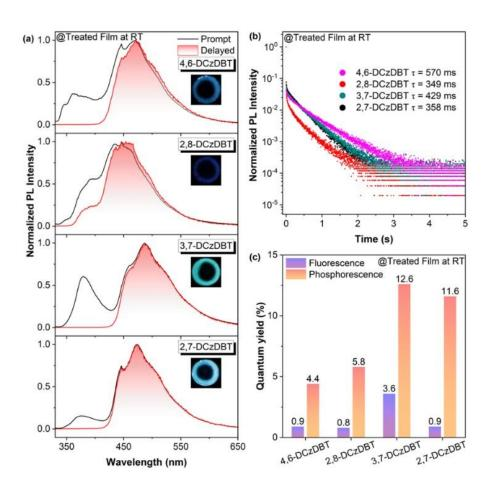
Figure 2 | (a) Normalized PL spectra and delayed (1 ms) spectra, (b) time-resolved phosphorescent decay curves, and (c) fluorescence and phosphorescence quantum yields under ambient conditions of treated PVA films with doped 4.6-DCzDBT, 2.8-DCzDBT, 3.7-DCzDBT, and 2.7-DCzDBT, Inset; photographs taken after the removal of the UV excitation source of 254 nm under ambient conditions of treated PVA films.
