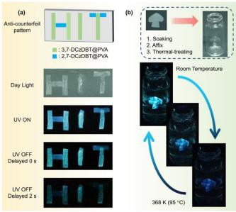
**Figure 7** | (a) Schematic diagram in preparation of anti-counterfeiting patterns and photographs of the security code before and after turning off the 254 nm UV lamp. (b) Schematic diagram in preparation of thermosensitive glasses with 3,7-DCzDBT film and pictures of thermal-sensing process from 368 K to 295 K under 254 nm UV lamp excitation
