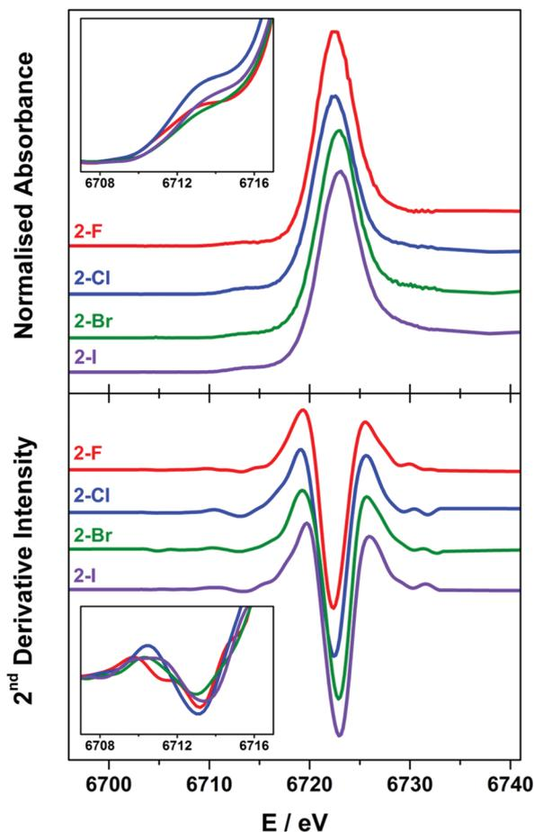
Fig. 6 Comparison of the normalised Sm  $L_3$ -edge XAS (top) and their FFT-smoothed second derivative spectra (bottom) of the 2-X (X = F, Cl, Br, and I) series recorded at 100 K. The insets show the expansion of the overlaid FFT-smoothed pre-edge peaks (top) and their second derivatives (bottom).
