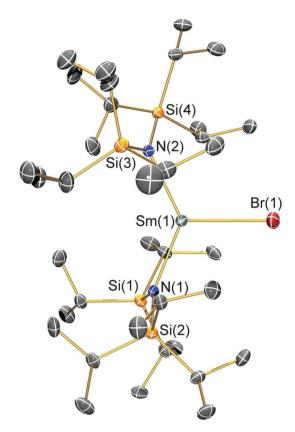
**Fig. 3** Molecular structure of  $[Sm(N^{\dagger\dagger})_2(Br)]$  (**2-Br**) with selective atom labelling. Displacement ellipsoids set at a 30% probability level and hydrogen atoms are omitted for clarity. Selected bond lengths [Å]: Sm(1)-Br(1) 2.7429(7), Sm(1)-N(1) 2.308(4), and Sm(1)-N(2) 2.324(4). Selected bond angles [°]: N(1)-Sm(1)-N(2) 133.52(14), N(1)-Sm(1)-Br(1) 112.19(10), and N(2)-Sm(1)-Br(1) 113.19(10).
