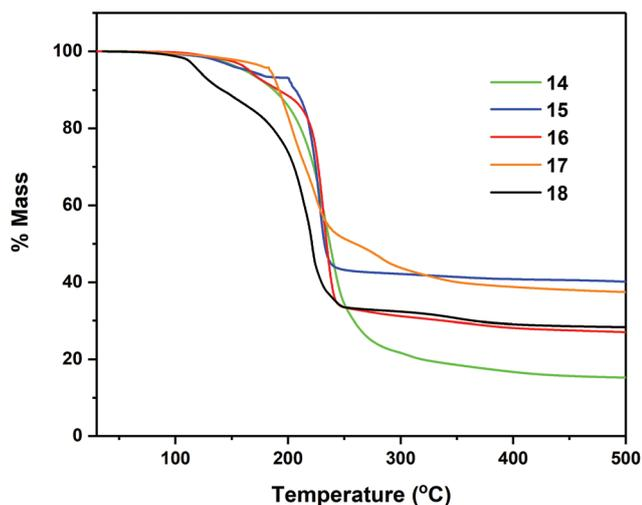
Fig. 10 Thermogravimetric analysis data for complexes 14–18.
