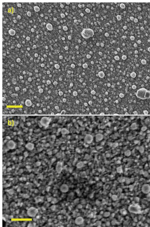
Fig. 11 SEM micrographs of Sn films deposited onto silicon substrates at 400 °C using precursors **6** (a) or **7** (b) respectively. Scale bar = 1  $\mu\text{m}$ .
