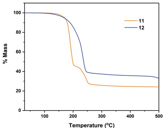
Fig. 9 Thermogravimetric analysis data for complexes 11–12.
