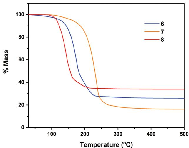
Fig. 8 Thermogravimetric analysis data for complexes 6–7.
