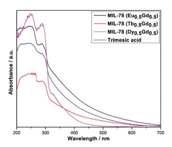
Fig. 5 UV absorbance spectra of MIL-78 (Ln $_{0.5}$ Gd $_{0.5}$ ); Ln = Eu, Tb, and Dy and trimesic acid.
