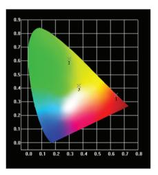
Fig. 7 1931 CIE chromaticity diagram of MIL-78 (Eu<sub>0.5</sub>Gd<sub>0.5</sub>) (1),  $(Tb_{0.5}Gd_{0.5})$  (2), and  $(Dy_{0.5}Gd_{0.5})$  (3).
