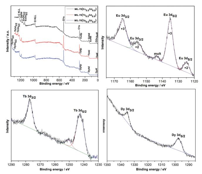
Fig. 3 X-ray photoelectron spectrum survey and narrow scans of Eu-3d, Tb-3d, and Dy-3d regions for MIL-78 (Ln<sub>0.5</sub>Gd<sub>0.5</sub>) Ln = Eu (black), Tb (red), and Dy (blue).
