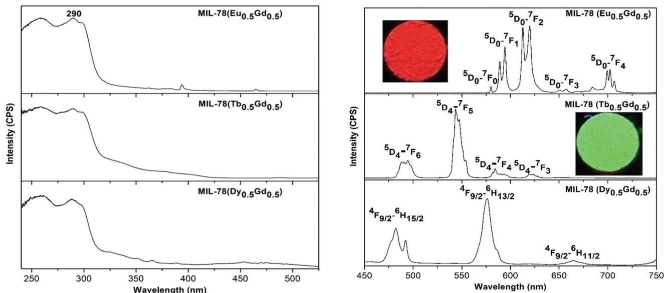
Fig. 6 Excitation (left) and emission (right) spectra of MIL-78 ( $\text{Ln}_{0.5}\text{Gd}_{0.5}$ ) with  $\text{Ln} = \text{Eu}, \text{Tb},$  and  $\text{Dy}$  at room temperature. The insets are showing the samples under UV light.
