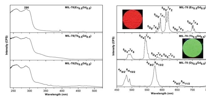
Fig. 6 Excitation (left) and emission (right) spectra of MIL-78 ( $Ln_{0.5}Gd_{0.5}$ ) with Ln = Eu, Tb, and Dy at room temperature. The insets are showing the samples under UV light.
