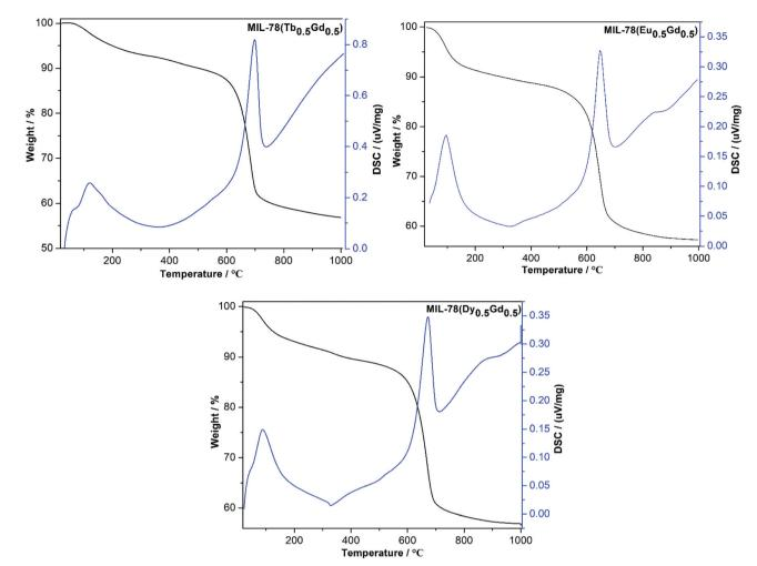
Fig. 2 TG (black line) and DSC (blue line) curves of the as-prepared MIL-78 ( $Ln_{0.5}Gd_{0.5}$ ) Ln = Tb, Eu, and Dy.
