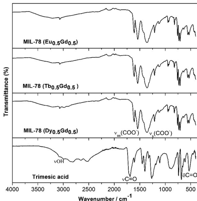
Fig. 4 Infra-red spectra of the as-prepared MIL-78 ( $\text{Ln}_{0.5}\text{Gd}_{0.5}$ ); Ln = Eu, Tb, and Dy and trimesic acid.
