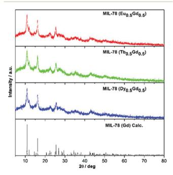
**Fig. 1** Powder X-ray diffraction patterns of the mechanochemically prepared MIL-78 ( $Ln_{0.5}Gd_{0.5}$ ) Ln = Eu, Tb, and Dy and the calculated pattern of MIL-78 (Gd).
