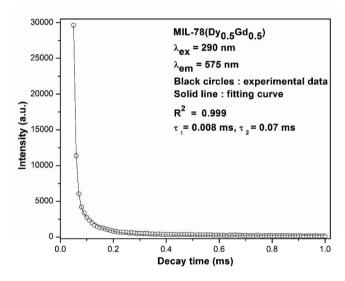
Fig. 8 Room temperature luminescence decay curves of MIL-78 (Ln<sub>0.5</sub>Gd<sub>0.5</sub>) Ln = Eu, Tb, and Dy.
