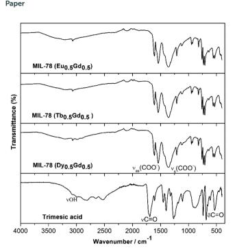
Fig. 4 Infra-red spectra of the as-prepared MIL-78 ( $Ln_{0.5}Gd_{0.5}$ ); Ln = Eu, Tb, and Dy and trimesic acid.
