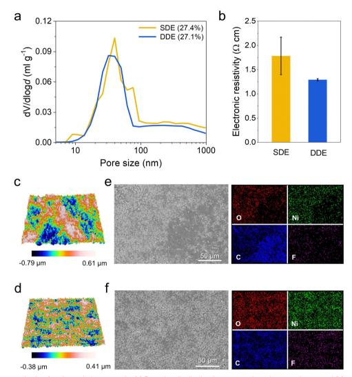
Fig. 2 Physical characterization for electrode homogeneity (a) Pore size distribution by mercury-intrusion porosimetry and (b) volumetric electronic resistivity of SDE and DDE. Surface roughness images showing electrode uniformity of (c) SDE and (d) DDE (338  $\mu$ m  $\times$  283  $\mu$ m). Top-view SEM images and corresponding EDS elemental mapping images of (e) SDE and (f) DDE.
