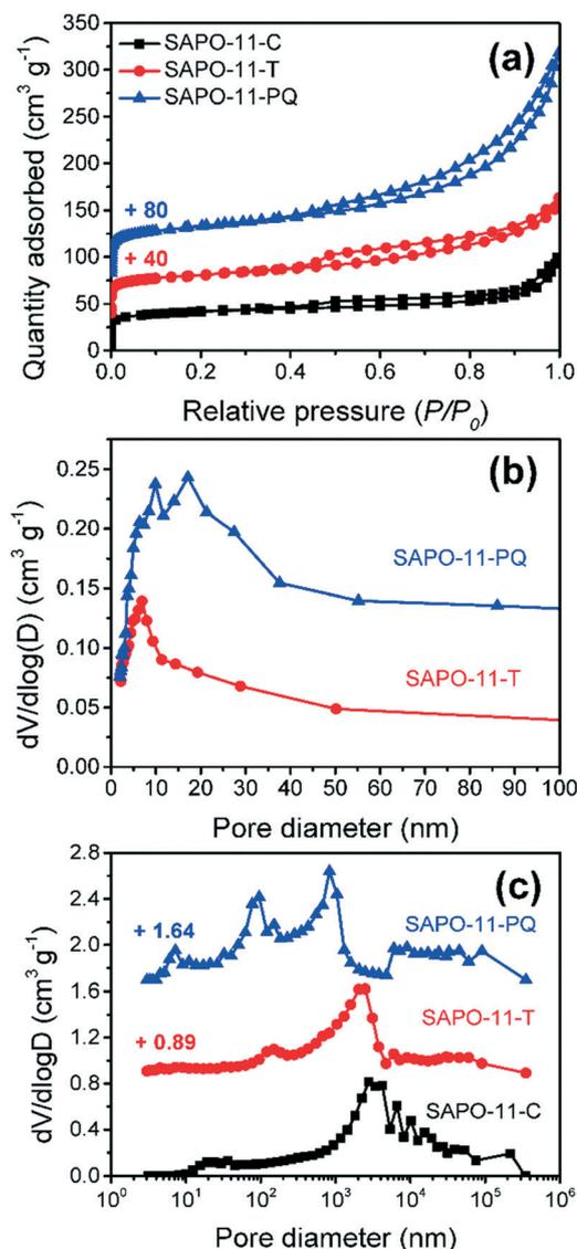
Fig. 3  $\text{N}_2$  adsorption/desorption isotherms of all samples (a) and the corresponding pore size distribution for all samples (b). Mercury intrusion based pore size distribution of SAPO-11-C, SAPO-11-T and SAPO-11-PQ (c).
