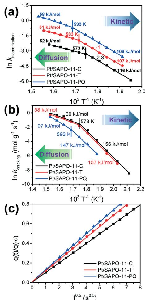
Fig. 8 Arrhenius plot of the *n*-heptane hydroconversion (shift down by a factor of 1 and 2.3 for Pt/SAPO-11-T and Pt/SAPO-11-PQ, respectively) (a), Arrhenius plot of the formation rate for stoichiometric propane and isobutene (b) and adsorption rates of 2-methylhexane in the calcined SAPO-11 samples (c).
