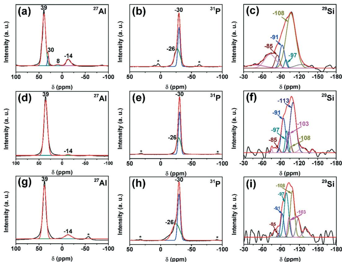
Fig. 4 <sup>27</sup>Al, <sup>31</sup>P and <sup>29</sup>Si MAS-NMR spectra of calcined samples: (a, b and c) SAPO-11-C, (d, e and f) SAPO-11-T and (g, h and i) SAPO-11-PQ.
