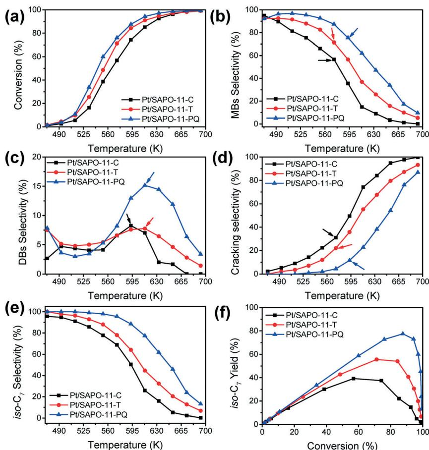
Fig. 7 Reactant conversion *versus* temperature (a), selectivity to MBs (b) and DBs (c) *versus* temperature, cracking selectivity *versus* temperature (d), total isomerization selectivity *versus* temperature (e) and total isomerization yield *versus* conversion (f). The arrows point to the maximum selectivity to DBs.
