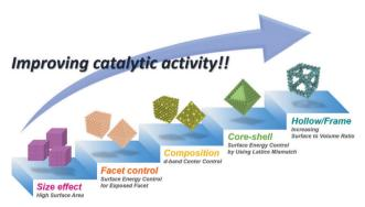
Fig. 7 Schematic illustration of brief history of the development of Pt-based ORR electrocatalysts (modified from ref. 5. Copyright 2016 AAAS).
