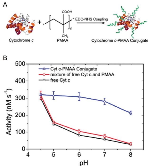
Fig. 2 Engineering pH-activity profiles. (A) Poly(methacrylic acid) modification of cytochrome C. (B) The pH-activity profile of cytochrome C towards the oxidation of Amplex Red in the presence of hydrogen peroxide. The negatively charged polymer shell around cytochrome C maintains a low local pH resulting in higher activity in more alkaline solutions. Reproduced with permission from *ACS Catal.*, 2017, 7(3), 2047–2051. Copyright 2017, American Chemical Society.<sup>34</sup>
