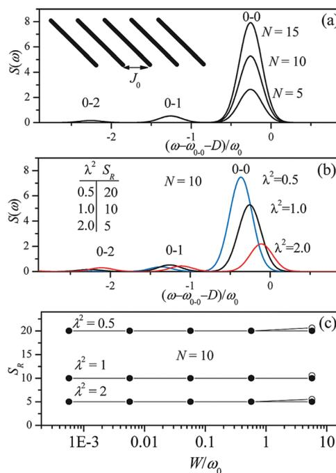
Fig. 1 Changes in the fluorescence spectra as a function of (a) the number of subunits  $N$  and (b) Huang-Rhys factor  $\lambda^2$ . Exciton bandwidth is set  $W = \omega_0 = 1400\text{ cm}^{-1}$  in (a) and (b). (c) Fluorescence vibronic peak ratio  $S_R$  as a function of exciton bandwidth. Adapted from ref. 8 with permission. Copyright 2011 American Chemical Society.
