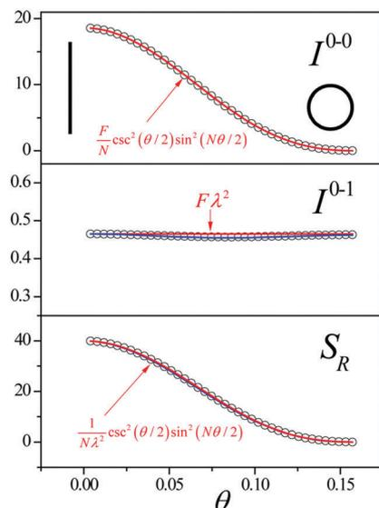
Fig. 2 Change in the 0–0 (top) and 0–1 (middle) fluorescence vibronic peak intensities, and the ratio  $S_R$  (bottom) as a function of curvature  $\theta$ .  $N = 40$  and  $J_{n,n+1} = -200 \text{ cm}^{-1}$  were used. Adapted from ref. 9 with permission. Copyright 2014 American Chemical Society.
