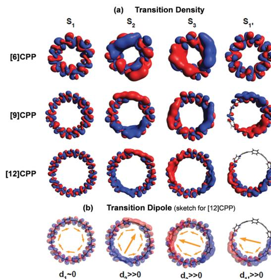
Fig. 5 (a) Transition density and (b) transition dipole moment of cycloparaphenylene 6-, 9-, and 12-mers at  $S_1$ ,  $S_2$ ,  $S_3$ , and relaxed  $S_1'$  states. Adapted from ref. 34 with permission. Copyright 2014 American Chemical Society.
