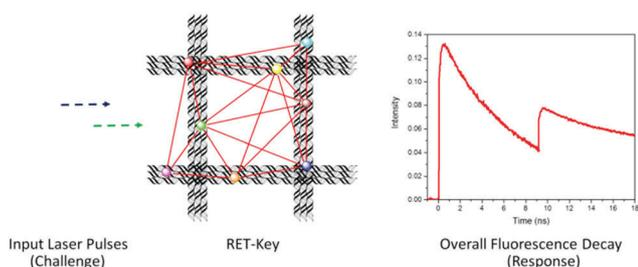
**Fig. 16** Schematic depiction of the RET-key function. Red lines in the RET-key indicate the cascade-like FRET processes between the appended fluorophores, allowing for a highly non-linear relation between the challenge and the response. Adapted from ref. 42.
