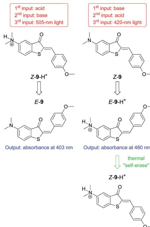
Fig. 11 Keypad lock function of the photoswitch **9**.
